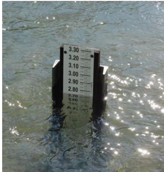
Photograph 3. Example of Typical Staff Gauge
